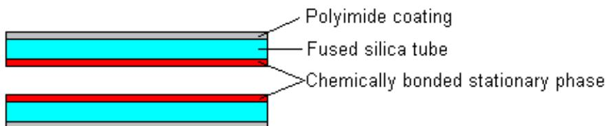
These have much thinner walls than the glass capillary columns, and are given strength by the polyimide coating. These columns are flexible and can be wound into coils. They have the advantages of physical strength, flexibility and low reactivity.
